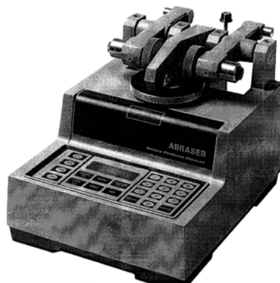
Fig. 1. Abrading instrument (vacuum not shown)
