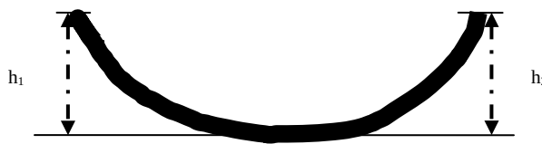
Figure 1. Curl measurement on a Forward Curl (F), where h_1 and h_2 are height of parallel edge of the specimen.
