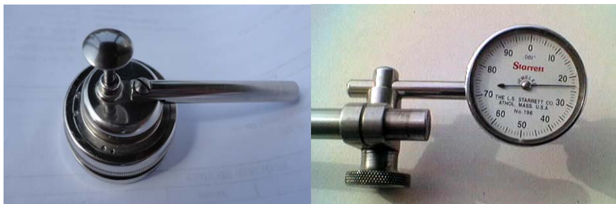
Fig. 2. Back-plunger style dial gage or indicator with "button" tip attached.
