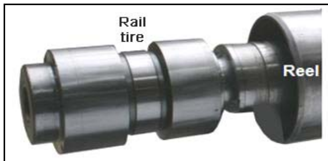
Figure 1. Typical reel spool journal, with size steps, drive connection (only on driven ends) and rail “tire.”
