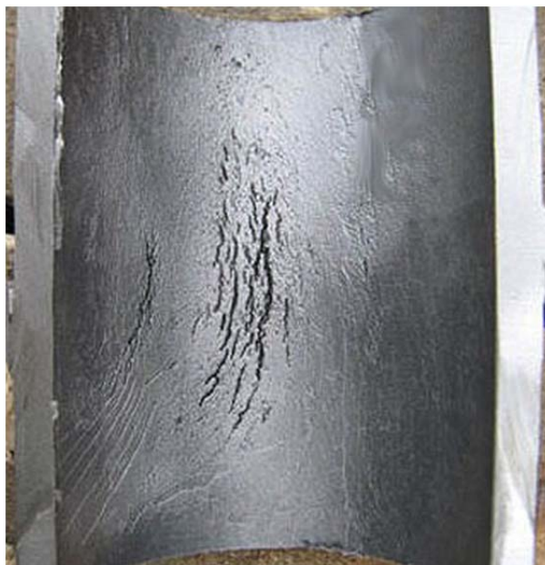
Fig. 1. Stress-assisted corrosion (SAC) damage in the internal surface of a 75 mm (3-in.) OD steel boiler tube with the scale removed to expose the crack-like damage.
