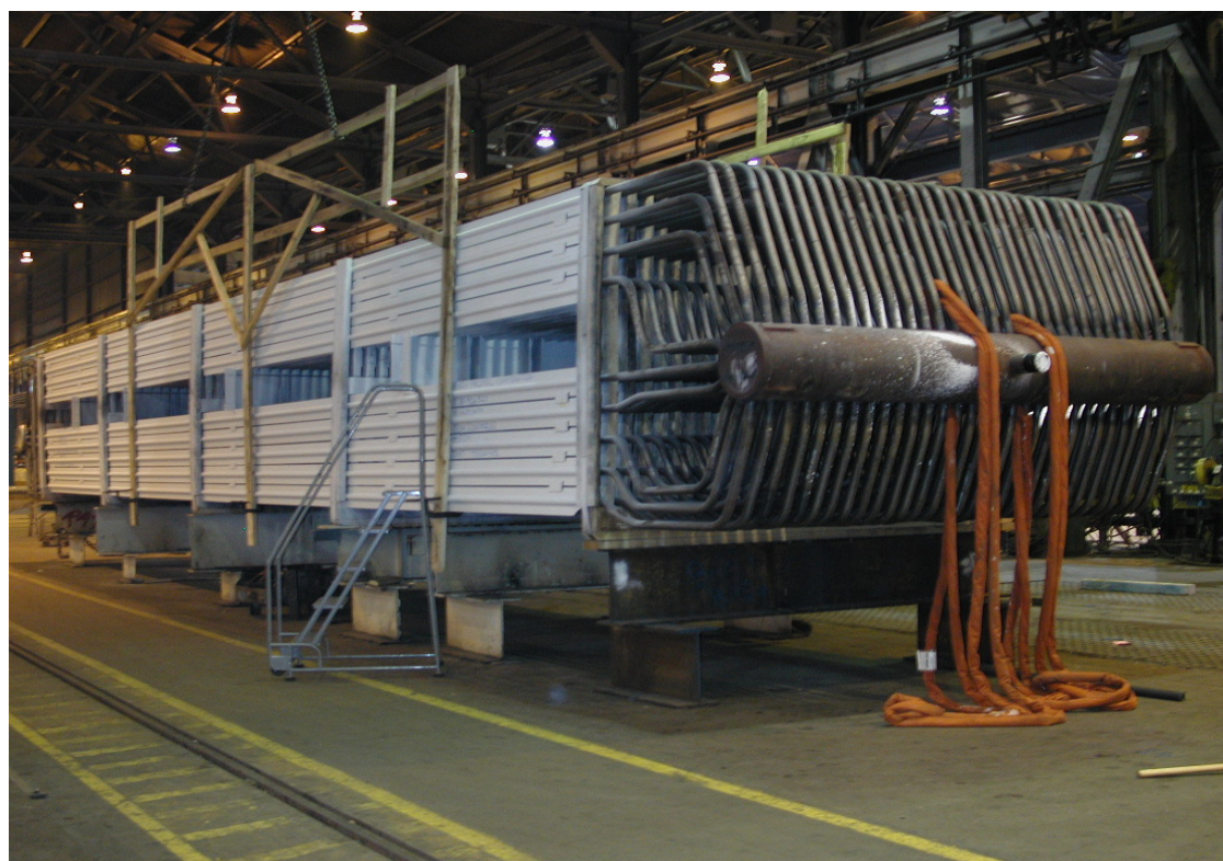
Fig. 3: Large header module
