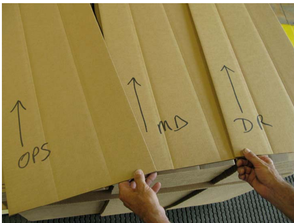
Fig. 1. Samples selected from operator, middle, and drive sides of corrugator.
