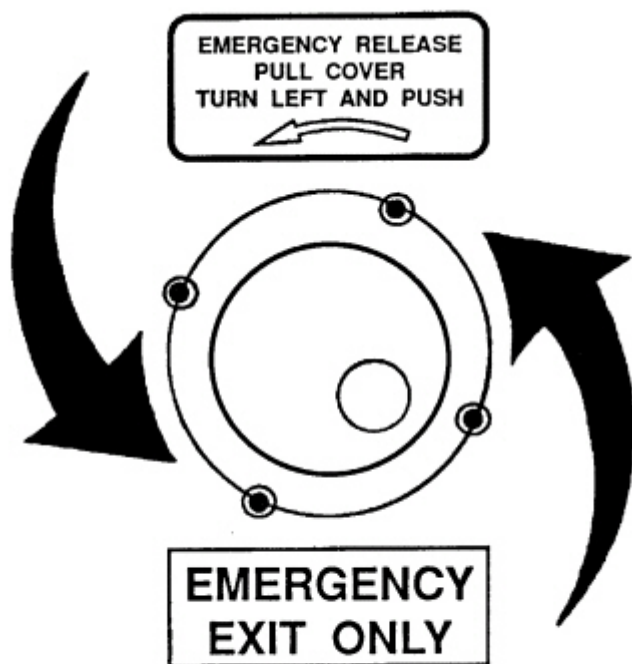
Figure 1. Approximate Installation of Arrows
