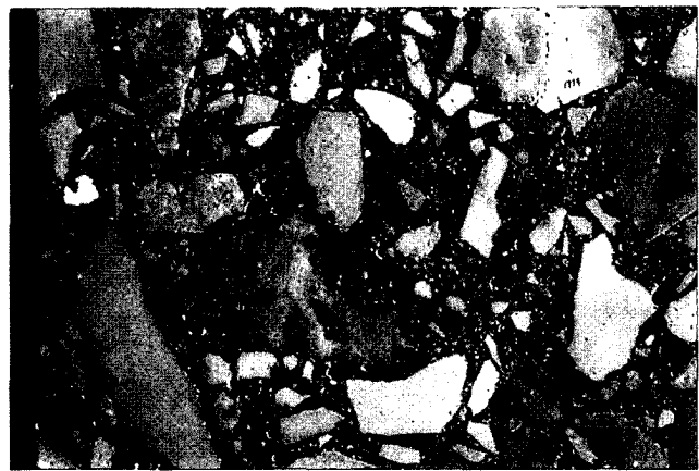
Fig. 2.7 — A polished cross section of concrete shows the aggregate, as the filler in the mixture, bonded together by the cement paste.
