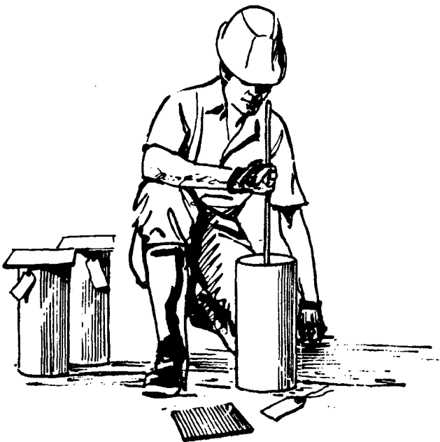
Fig. 2.4 — Concrete test cylinder molds are filled with fresh concrete in three equal layers, each layer being rodded 25 times. Each cylinder should be labeled and capped or otherwise protected to prevent loss of moisture.
