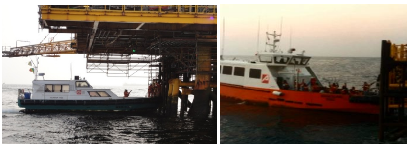
Figure 1 – Transfer of personnel using ‘Surfer/Mamolino’ type crew boat
