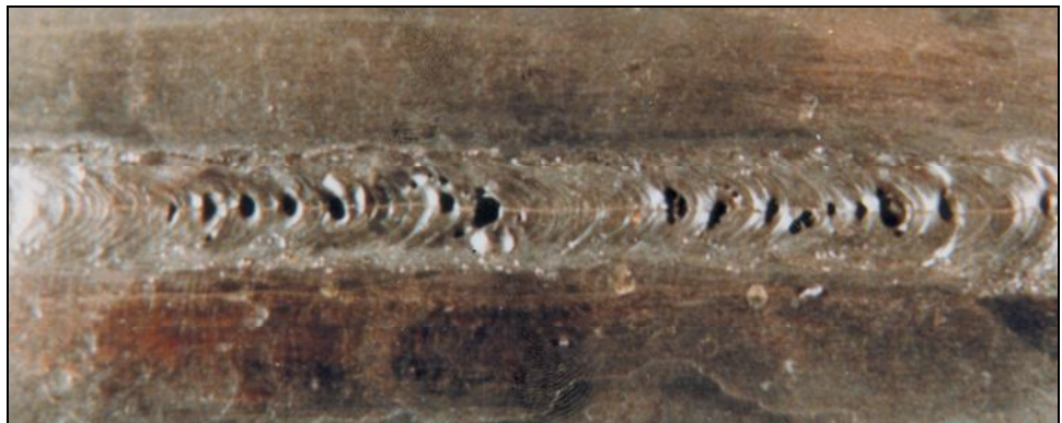
Figure 2.3—Aligned Porosity with Crack
