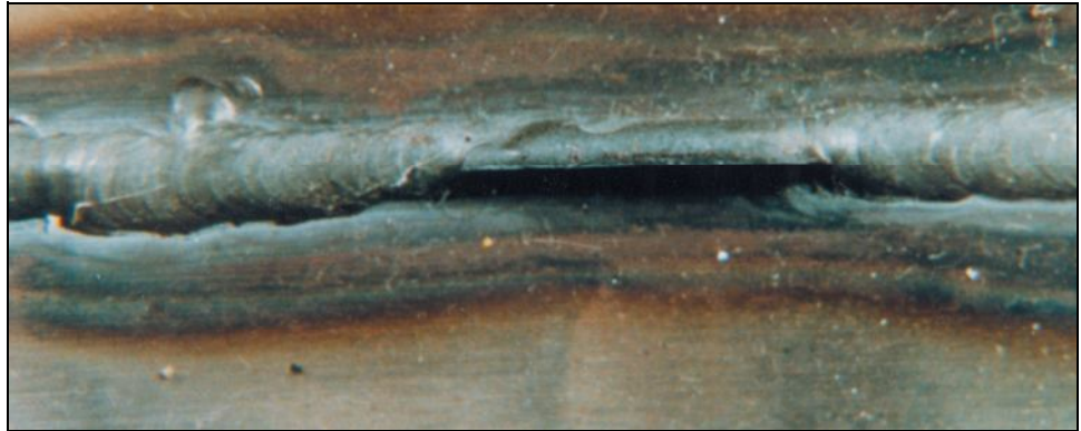
Figure 2.11—Incomplete Joint Penetration with Consumable Insert
