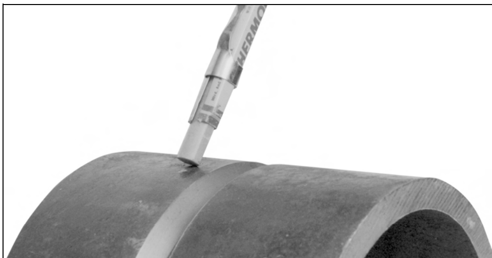
Figure 1.3—Using a Temperature Indicating Crayon
