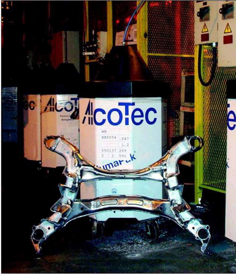
Figure 1.3—Fabricated Aluminum Engine Cradle
