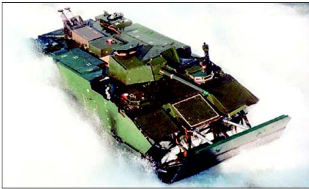
Figure 1.15—The Corrosion Resistance and Light Weight of Aluminum Allows this Military Amphibious Vehicle to Travel at High Speeds on Land and Over Water
