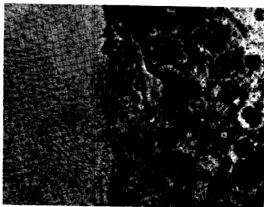
4 HAZ cracking, using austenitic stainless steel filler ( \times 100 )
