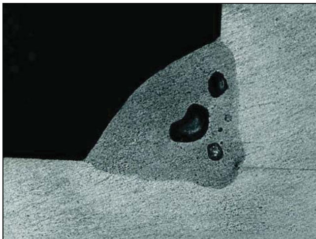
Figure 1.4—Porosity in a Cross Section of a Fillet Weld in Aluminum
